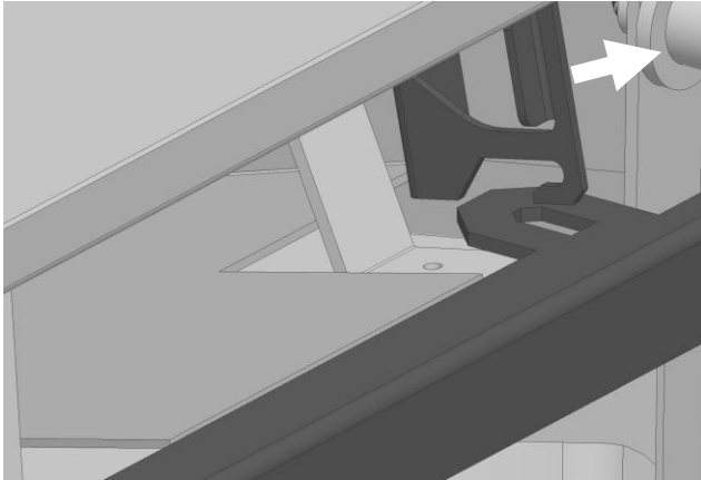
Figure 13 – Glass Frame Upper Mounting Detail
