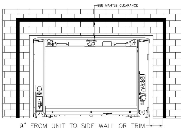
Figure 17 - Minimum Side Trim Clearances
